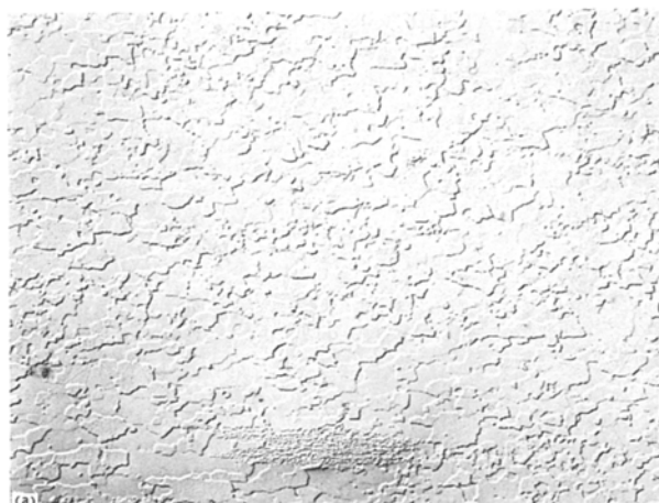
Figure 5 Examples of recrystallization found in specimens tested at 1300 K and a strain rate \approx 2 \times 10^{-5} \text{ sec}^{-1} to \sim 10 strain: (a) NiAl-0.5HfC and (b) NiAl-4.3HfC. Compression axis is horizontal; specimens etched with a mixture of 33 HNO 3 , 33 acetic acid, 33 H 2 O, and 1 HF (vol %). Photomicrographs taken under differential interference conditions; disruptions in part (b) are large HfC particles.
